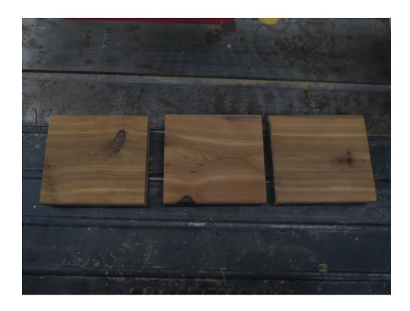
From the remaining board cut four 9" sections. In each of these four sections cut a  $\frac{1}{2}$ " notch along the long dimension. These notches will be used to make half-lap joints for the roof. The peak will be a square butt joint.
