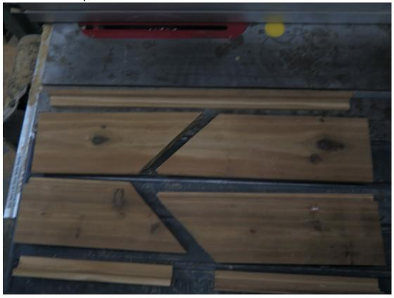
The single notched 22" section will make the sides, joined with one of the trim edges from the back. Square both ends. Cut two 10" lengths. Using the trim saved in the previous step cut two 10" pieces. These will be joined to make the sides a little wider to accommodate standard sized nesting tubes.
