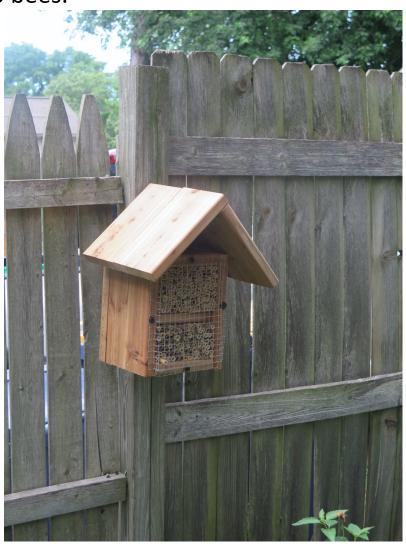
Made from one  $5/4 \times 6'' \times 10'$  cedar deck plank (actual dimensions are  $1'' \times 5 \frac{1}{2}'' \times 10'$ ).
