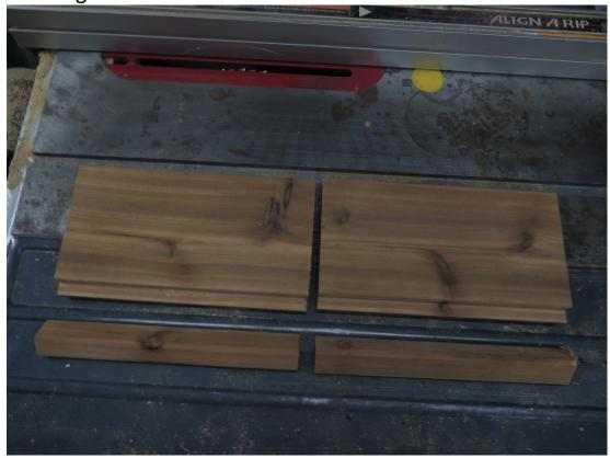
From the remaining board cut three 6" pieces for the top, middle, and bottom of the bee hotel. When installed these will be flush with the front edges of the sides, with a small gap at the back. Alternately you can notch these sections and use the remaining notch section from the back to make them the same length as the sides.
